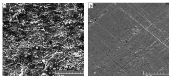
Fig. 7: SEM images of mild steel specimens in a HCl, b HCl with 100 mg/L of inhibitor.
